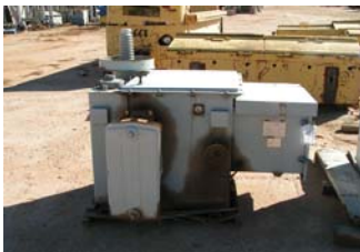
NWL Transformer/Rectifier, 80.2 KVA
