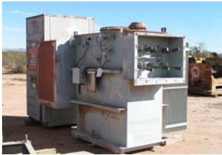
Virginia Transformer, 1000KVA w/ load interruptor switch
