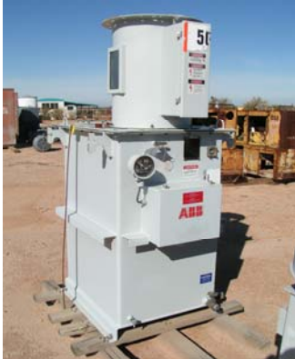
ABB Transformer/Rectifier, 58.9 KVA
